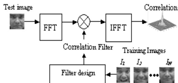
Figure 1. Block diagram showing the correlation process
