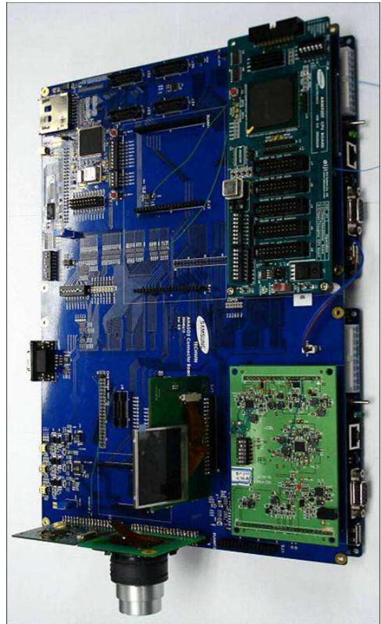
Figure 1: Initial Samsung FPGA DSC Platform using S5C7380x
