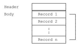
Figure 6: Structure of a cyclic file
