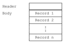
Figure 5: Structure of a linear fixed file
